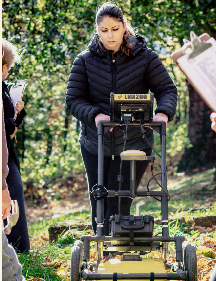
Dr. Sarah Beaulieu conducting ground penetrating radar
